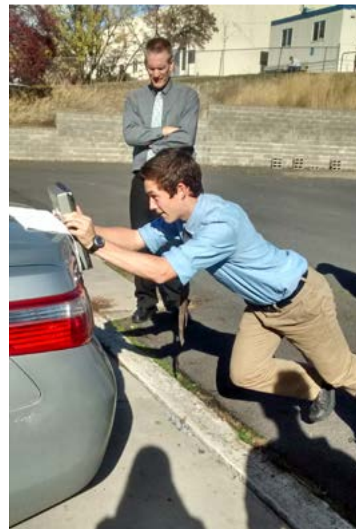
Mr. Loren Euhus looks on as Drew Pilchard notes, by pushing on a scale, the force necessary to move a particular car a particular distance.
